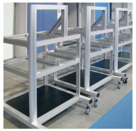
Mobile support frame built from Series 40 cleanroom profiles
