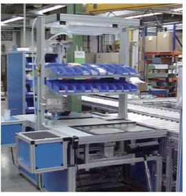
Industrial workstation in DFT flow line for manufacturing vacuum pumps
