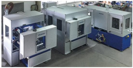
Extendible guarding elements; sections mounted on rollers can be moved manually over the first section
