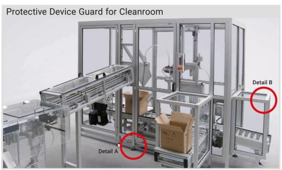
Protective device guard for applications in the cosmetics industry. Because of the stringent sanitary requirements, the machine housing was built from Series 40 cleanroom profiles with closed profile slots. Scratch-resistant Makrolon was used as the panelling material to provide an unobstructed view of the packaging station. Stainless steel levelling feet were also used, which are ideal for the conditions mandated by the sanitary regulations.
