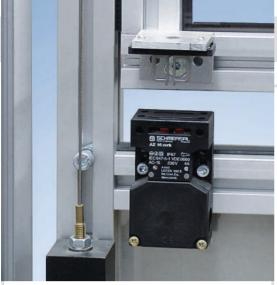
The switching element and actuating keys for the safety interlocks are not connected to each other, but are functionally combined or separated when switching. The actuating key is separated from the basic device when the guarding is opened. In doing so, the normally closed contacts are opened and the normally open contacts are closed in the safety interlock.
