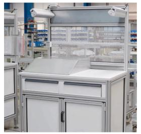
Test station made from Series 50 profiles, base cabinet with drawers and swing door, gantry with steel and perforated sheet panelling
