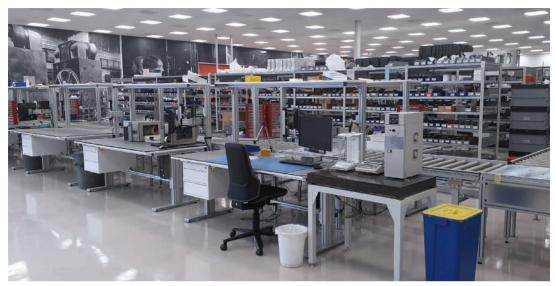
ESD-compliant assembly and test line with integrated conveying path for analysis units
