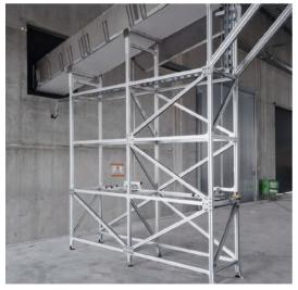
Frame and suspension for conveying path at a height of 5 m below the hall ceiling
