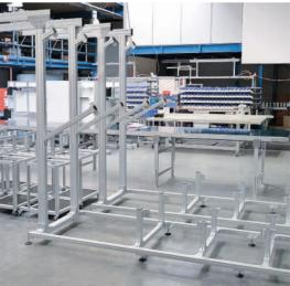
Frame for hopper conveyor made from Series 50 profiles
