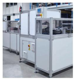
Protective device guard with interlocked swing doors for removal and inspection of the component
