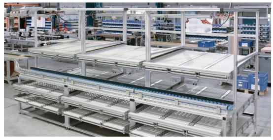
Kanban system workstation for manual removal and picking of products
