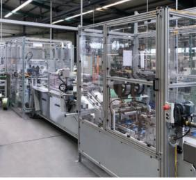
Retrofitting of a production line with protective device guards
