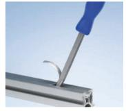
Parting Tool for Cleanroom Profiles
