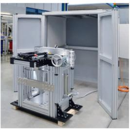
Protective housing for balancing stand, access via swing door with safety interlock and safety controller for the balancing stand
