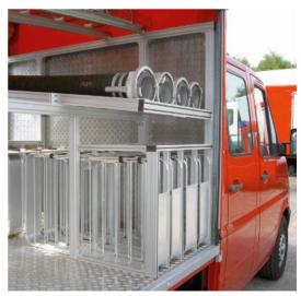
Fire engine interior built from Series 25 profiles
