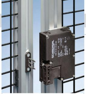
Protective doors that are secured with solenoid latches are generally only opened in exceptional cases. Solenoid latches use electric magnets to activate an interlock, which blocks or triggers the actuating key of the switch.
