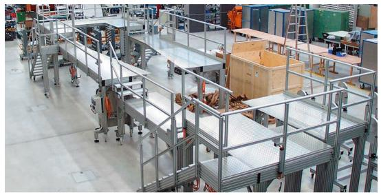
Free-standing assembly platform, 15 metres long, with high-load stairs for secure grip when carrying heavy loads
