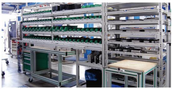
Kanban workstation for increasing productivity by decoupling assembly and supply logistics
