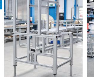
Machine frame made from Series 50 profiles
