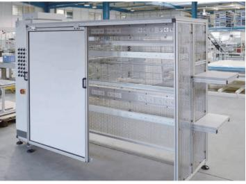
Test station for pumps with perforated sheet panelling, sliding door and keyboard shelves
