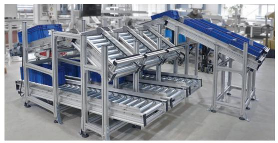
ESD-compliant loading and unloading station for feeding of small load carriers
