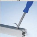
For cutting or exposing slots (10 mm in cleanroom profiles.
