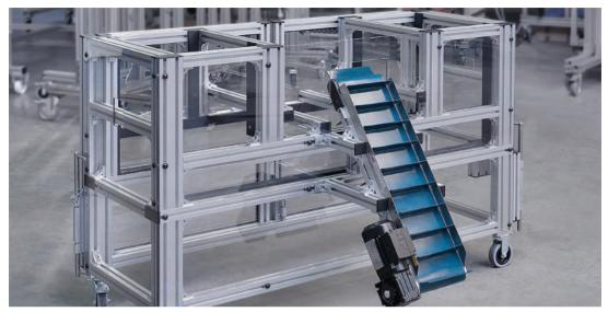
Mobile frame with double swing door and integrated belt conveyor made from Series 40 profiles
