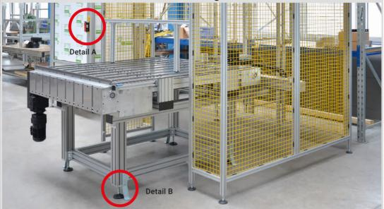
The system's gripping and transfer station is safeguarded using panel frames with welded grids in a custom RAL colour all around the station. The in-feed area and the measuring cell are protected by panel frames with polycarbonate and cover panels. A space-saving folding door is installed in addition to the swing door.
