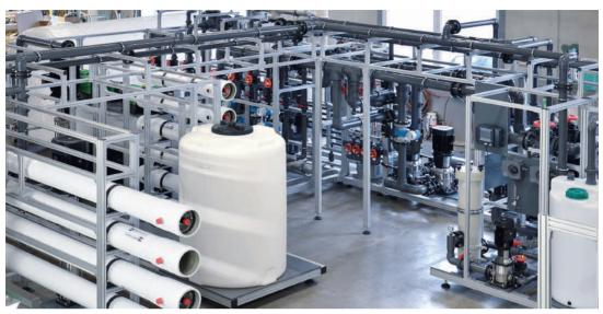
Flexible light-duty frame made from Series 40 profiles for desalination plant
