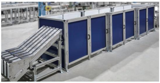
Soundproof enclosure with double swing doors and with convoluted foam cover for coin transport system
