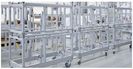
Testing and storage frame for fuel tanks made from Series 40 profiles
