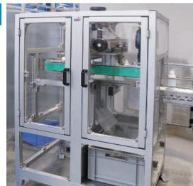
Guarding with swing doors made from cleanroom profiles
