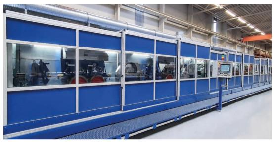
Mobile machine housing using Series 50 profiles for strip rolling line
