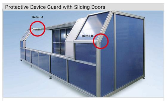
A machine housing was built for a manual lathe. The shape and appearance of the guarding needed to be adapted to the lathe. The housing was completely closed off using sheet panels to prevent chips and drilling fluid from getting into the production hall. Two separately controlled sliding doors allow easy access and operation of the machine. Optionally, the sliding doors can be driven electrically using a timing belt.
