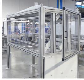
Charging unit for non-woven fabric production with maintenance door and extraction hood
