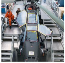
Mobile assembly platform for helicopters with different levels and multiple access points
