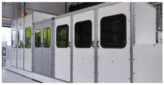
Protective laser enclosure with labyrinth seals for automation line
