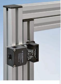
The switching element and actuating keys for the safety interlocks are not connected to each other, but are functionally combined or separated when switching. The actuating key is separated from the basic device when the guarding is opened. In doing so, the normally closed contacts are opened and the normally open contacts are closed in the safety interlock.
