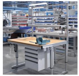
Workstation with electro-hydraulic height adjustment and base cabinet
