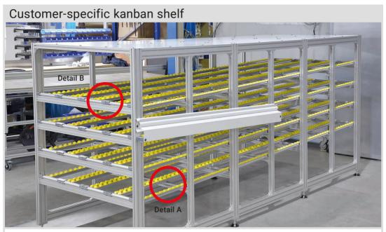
Here, support plates are removed from the kanban shelf according to the first-in-first-out principle. The empty support plates are returned vertically to save space. This kanban shelf is extra long to achieve the required storage volume. The frame is extremely solid so that it can safely hold the relatively high loads.
