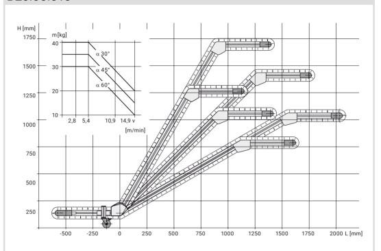
See the table for the optimal variant for your application. Without additional specifications, the conveyor is designed with a top, front left, 270° drive location and speed of 5.4 m/min.
