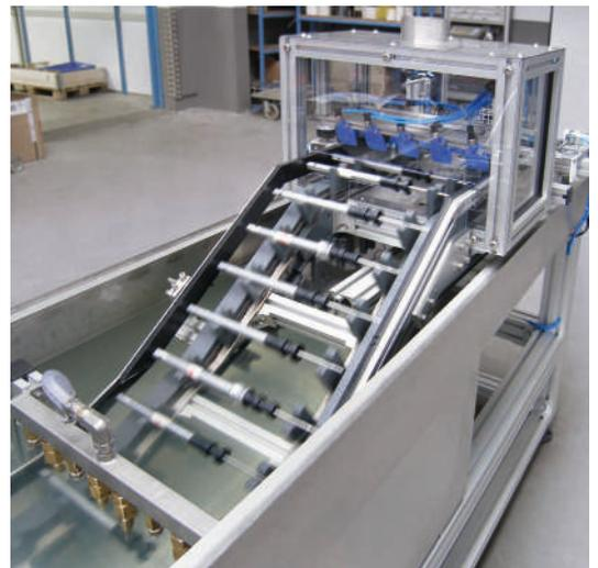
Customer-specific TKU 2040 with 20° inclination and transport of workpieces through a cleansing bath
