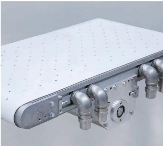
Vacuum belt conveyor GUF-P 2041 BC with 3 chambers in transverse direction for batches of paper envelopes of different widths
