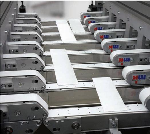
Vacuum belt conveyor made of stainless steel with knife edge for fast transport of fleece strips
